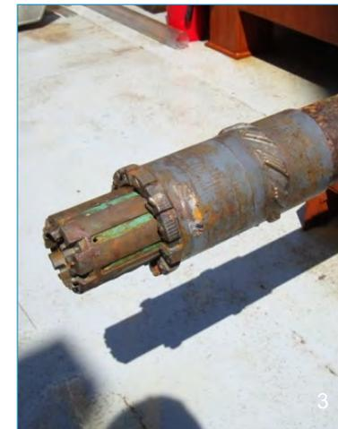
'Lighter' coring system, higher rotational speed, smaller gap between borehole wall and drill pipe, can lead to better hole condition and better core quality
